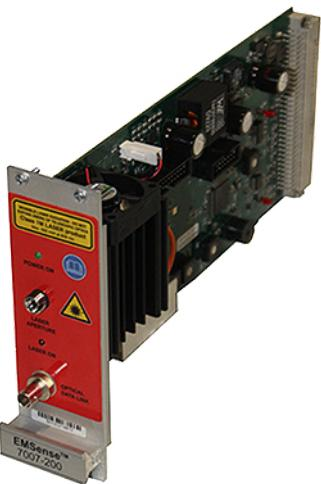
The **ETS-Lindgren EMSENSE™ 10/40 EMF Probe Plug-in Card** provides seamless power and communication to ETS-Lindgren's laser-powered electric field probes, ensuring reliable performance without the need for external power supplies. Designed for true plug-and-play operation, the card integrates directly with the EMCenter Modular RF Platform, simplifying setup and minimizing downtime.
