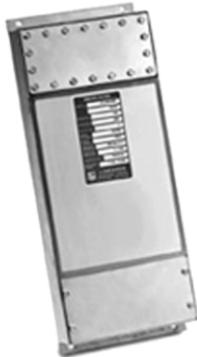
**ETS-Lindgren's LRW Series Single & Dual Line Filters** are UL Listed and come with mounting penetration and hardware for direct installation through a shielded wall. These filters are designed and manufactured to the most current version of UL-1283 and in accordance with the Low Voltage Directive (2006/95/EC) and IEC 60939. All LRW Series Filters meet or exceed 100 dB insertion loss from 14 kHz to 40 GHz as measured per MIL-STD-220C.
