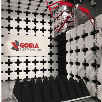
**ETS-Lindgren's FACT 3 EMC Anechoic Chambers** small overall size results from the use of hybrid absorber and ferrite tile, which require less volumetric space than traditional absorbers. ETS-Lindgren FACT 3 chambers will fit in many existing structures, yet are large enough to perform 4 meter antenna scans above the ground plane. When installed with ETS-Lindgren's LoPro™ or EuroPro™ turntables, pit excavations for motor assemblies are eliminated.
