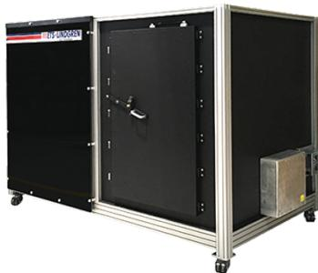
**ETS-Lindgren's AMS-5705 CATR 5G Antenna Measurement System** is an indirect far-field compact antenna test range (CATR) system with a 30 cm QZ. The system meets 3GPP and CTIA quality-of-quiet-zone and phase-validation requirements for 5GNR bands n257 through n262. AMS-5705 is also Qualcomm approved for FR2 beam characterization and verification. Its 30 cm QZ is perfect for 5G FR2-enabled smartphone and tablet testing with CTIA approved phantoms.
