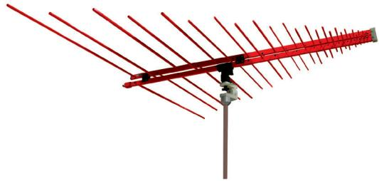
**ETS-Lindgren's Model 3144 Log-Periodic Dipole Array (LPDA) Antenna** is a standard medium gain (6 dBi) log-periodic dipole array. This log antenna is enables users to measure from 80 MHz to 2 GHz in one sweep, which saves time and money by eliminating the need for antenna changes at band breaks.
